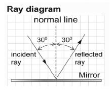
2. Use the law of reflection to draw the path of the reflected ray from the mirror in the diagram below.
