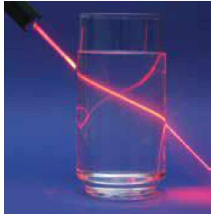
Figure 3.21: The beam of red light allows you to see the path of light bend as it enters and leaves the water.
