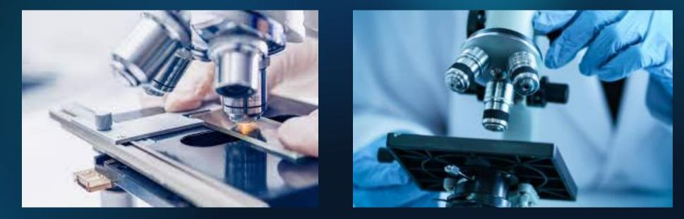
Never use coarse adjustment with high power lens.
